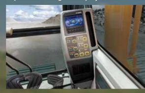
Instrument Panel is installed in front of RH console box. It is easy to check all critical systems with easy-to-read indicators.
