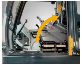
New joystick grips for precise control have been equipped with double switches. - Left: One touch deceleration - Right: Horn / Optional
