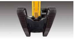
Reinforced box-section frame welded, low-stress, high-strength steel, guarantees safety and resistance against external impact when driving on rough ground and working on wet sites through high tensile strength steel panels, with highly durable upper and lower rollers and track guards.
