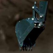
Sealed and adjustable bucket linkage provides less wear of pins and bushes as well as silent operation. The design includes bucket link durability and anti wear characteristics. Additional reinforcement plates on cutting edge section. Reinforced bucket is made with thicker steel and additional lateral plate.
