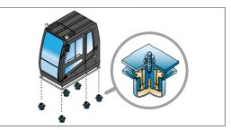
The application of Viscous Mounting to the cabin support provides the operator with a much improved ride. The operator work efficiency will increase as the shock and noise level in the cabin decreases.
