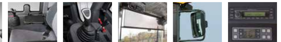
Wrist rest Joystick lever Front sunshade Side mirrors AM/FM Radio with MP3/ AC control
