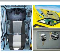
Wide, Comfortable Operating Space 2 Steel Cover Sunroof 3 Dial Type Engine Speed Switch and Key Switch
