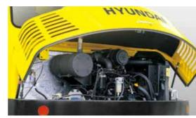
Easy to Maintain Engine Components The R80-7 was built with accessibility in mind. All doors, covers and hoods were built for complete open access. You'll find that the R80-7 offers plenty of space to complete your regular maintenance and service hassle-free.
