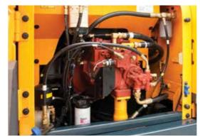
To achieve optimum precision, Hyundai redesigned the hydraulic system to provide the operator with super fine touch and improved controllability. Improved pump flow control reduces flow when controls are not being used to minimize fuel consumption.
